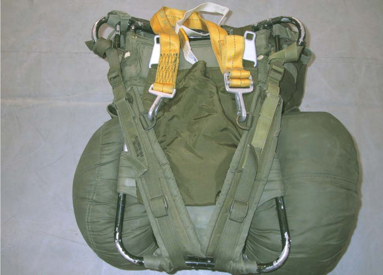
Figure 13-3: Jettison Buckle Routing
