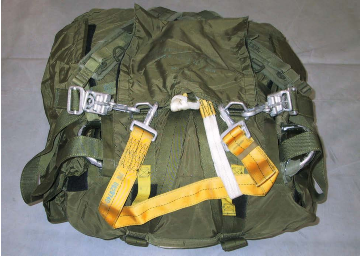
Figure 8-6: Jettison Strap Attachment
