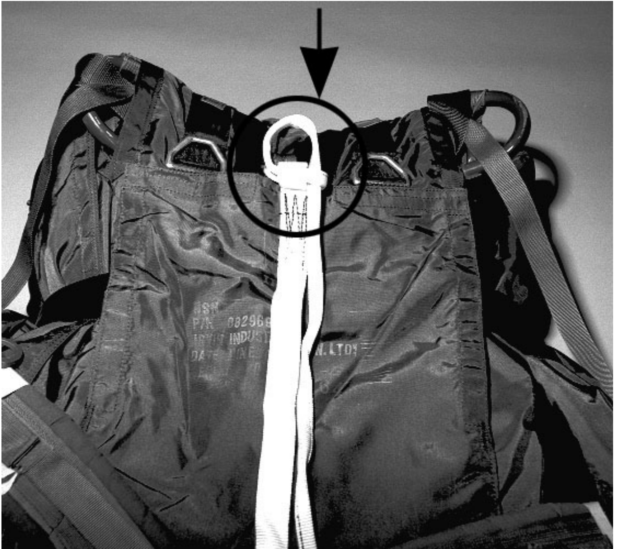
Figure 2-6: Thread Running End down through the Bight
