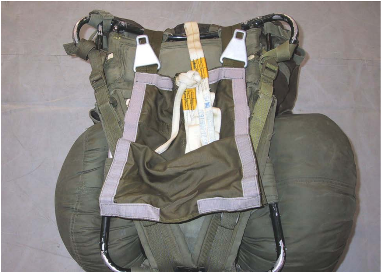
Figure 13-2: Lowering Strap Attachment
