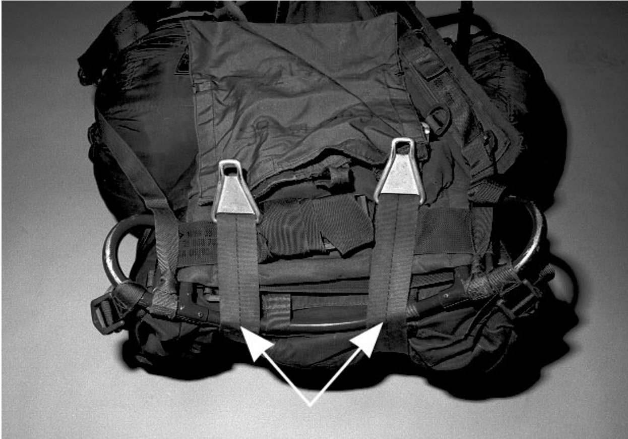
Figure 2-9: Routing PELS over Bottom Portion of Rucksack
