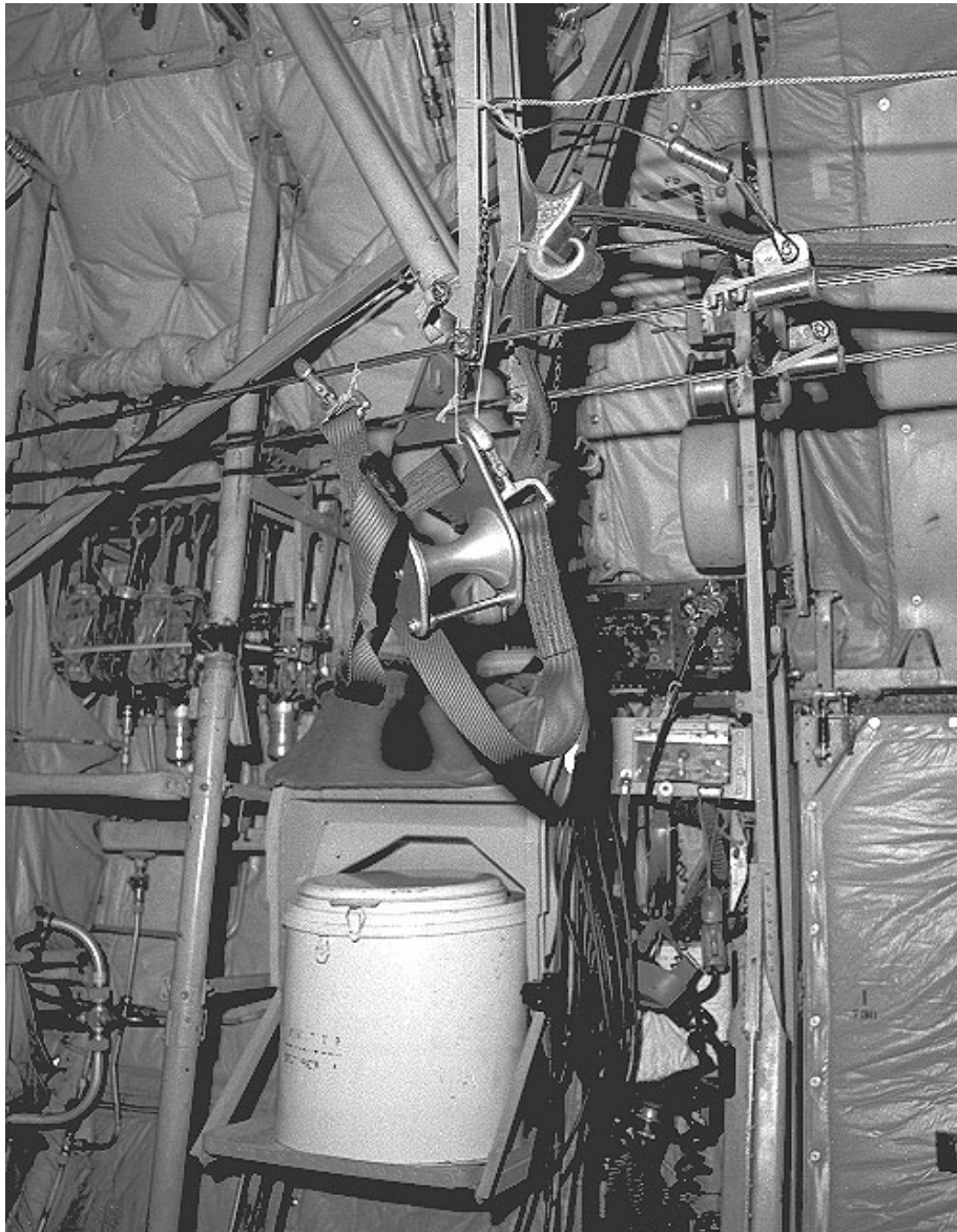
Figure 4-2: Retrieval Gear for a Door Exit.
